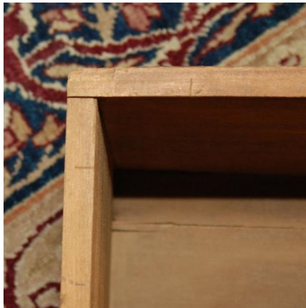
Figure 5. Chisel-punched marking system used by the maker S to differentiate left from right drawers with one or two chisel marks. This system is used on the NRF dressing table (above), the upper left and right drawers of the chest shown in Figure 1, and the same convention is used throughout the desk bearing the label of Job Townsend at the Rhode Island School of Design. Below: single chisel marks in the inner left rear corner of a chest drawer.
