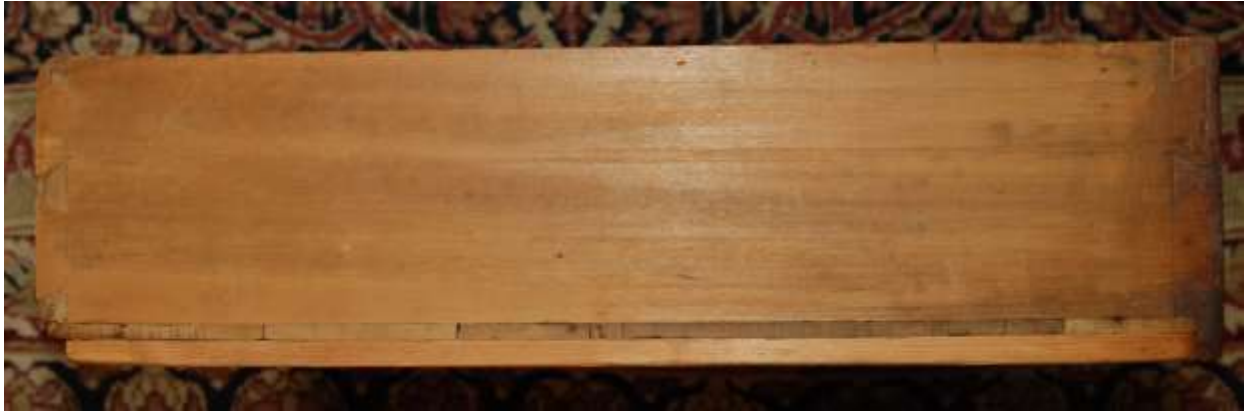
Figure 3. Drawer side from a Townsend chest showing the drawer side tail layout of two tails at each end. The front is at the right and the rear is at left. The sides and back are 3/8" thick and the tails are 7/16" long, resulting in some overhang at the back.
