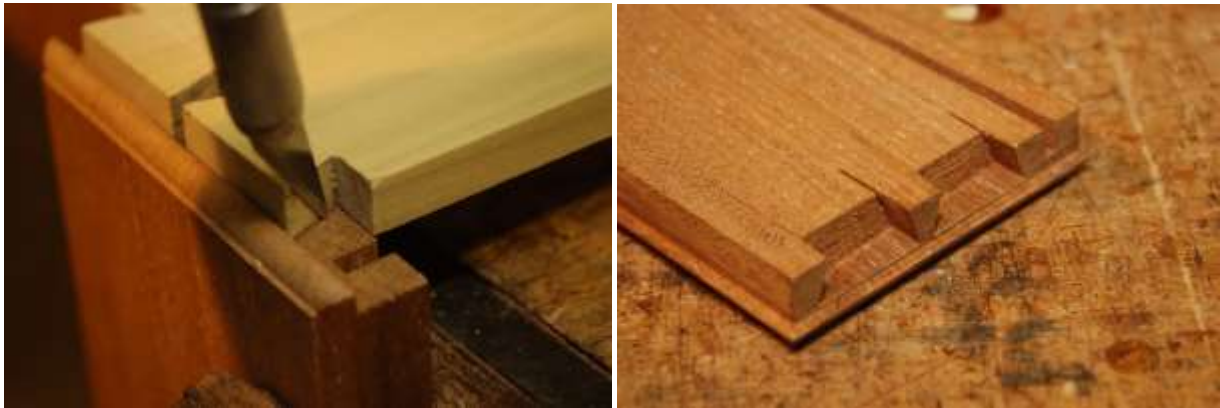
Figure 9. The pins are then scribed on the drawer front from the now-tapered tails (left) and the material between is sawn and chiseled away (right).
