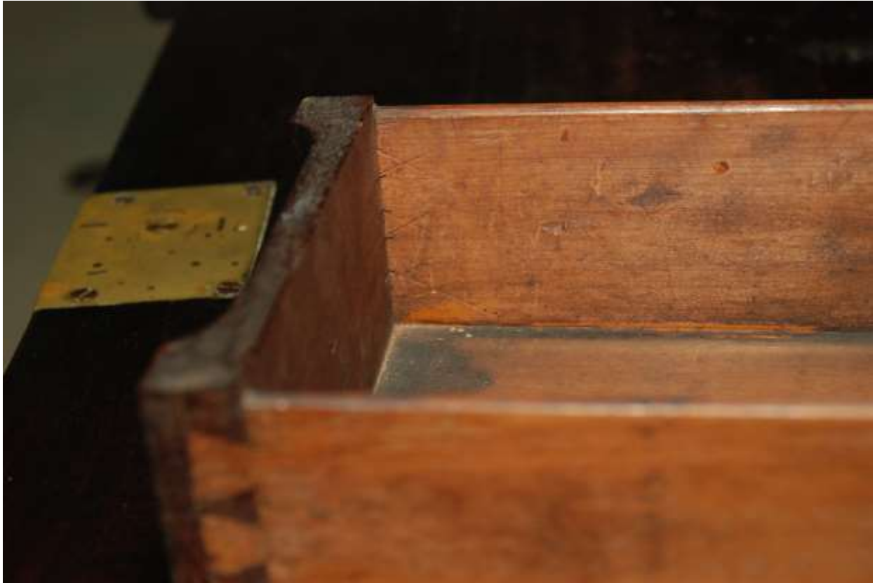
Figure 5. Interior of a desk drawer by an unknown Newport maker. Thick scribe lines inside the drawer lay out the tail positions which were then cut somewhat inaccurately. The pins were then scribed from the cut tails.
