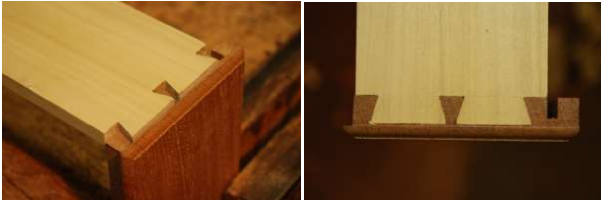
Figure 10. The joint now assembles easily by hand (left), but needs a block and mallet to be assembled fully (right). The resulting joint is very tight at the base of the tails with no damage to the delicate tips of the pins.
