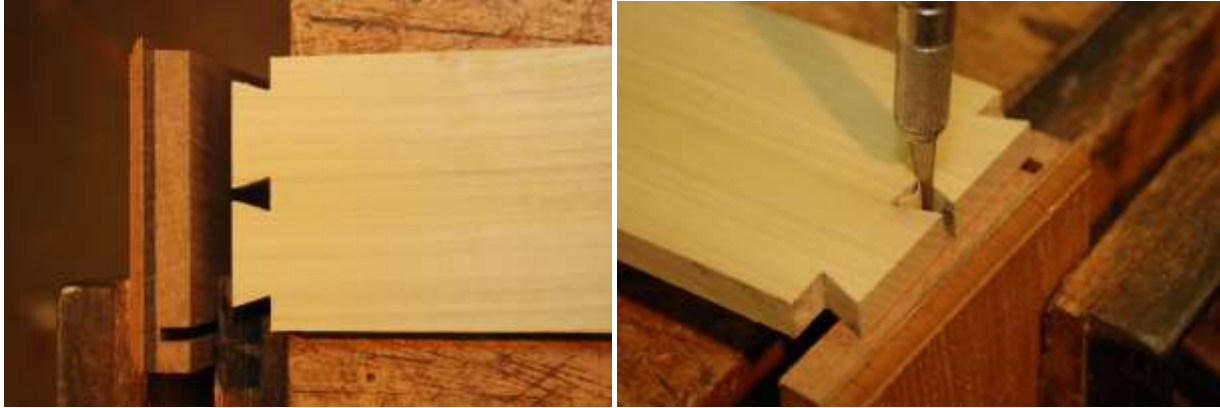
Figure 8. Tails are first laid out and cut (left), then the drawer side is turned over and slight tapers are cut on the inner faces of the tails (right). Note there is no taper at the tip of the tail and it increases toward the base of the tail. This taper is very slight, removing only about 1/64" on each tail face since the effect is additive with each tail.
