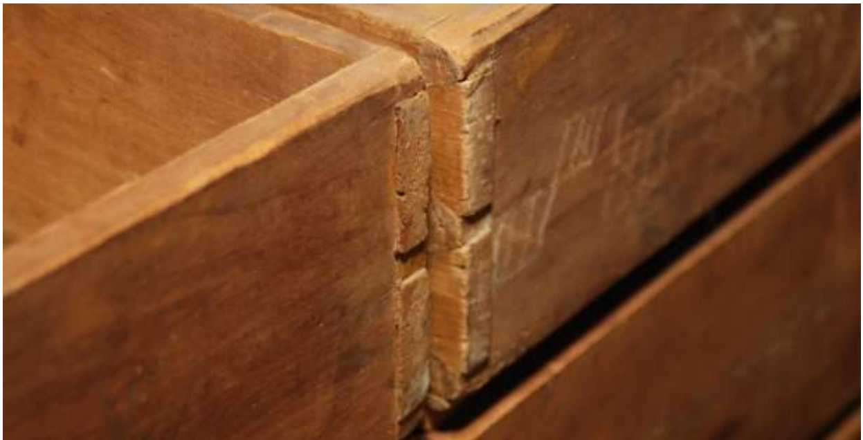
Figure 4. Close-up of the back of drawers of Townsend shop chest showing sides extending past the drawer backs. The sides were first scribed and cut for 7/16" long tails and therefore extend 1/16" beyond the 3/8" thick backs.
